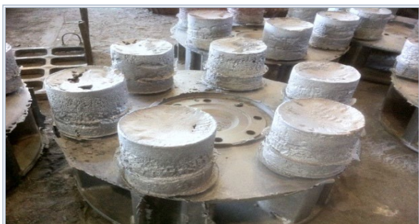
Figure 1. Six (10 in. x 12 in.) risers are shown as cast. (Artwork courtesy of Ebacero Foundry.)
