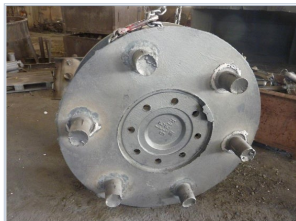
Figure 2. Six XL 2565 mini-risers on the rotor casting are shown. (Artwork courtesy of Ebacero Foundry.)
