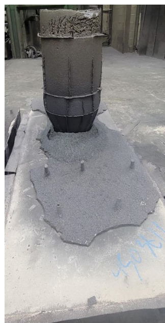
Figure 3. The casting with a large neck riser as cast showing burn-in from excess heat from the riser. (Artwork courtesy of The C.A. Lawton Co.)
