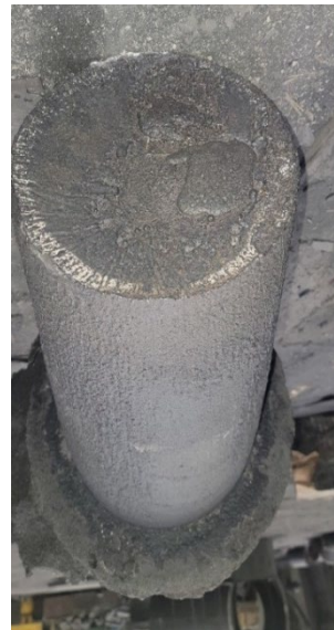
Figure 6. The resulting XL 26000 riser after removal from the casting which shows comparatively minimal burn in under the riser. (Artwork courtesy of The C.A. Lawton Co.)
